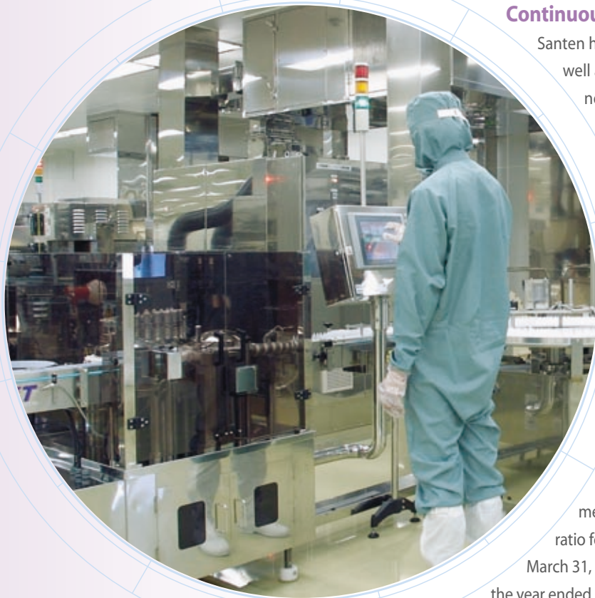
Inspection on the Dimple Bottle production line. The form of each container is checked by a computer.
